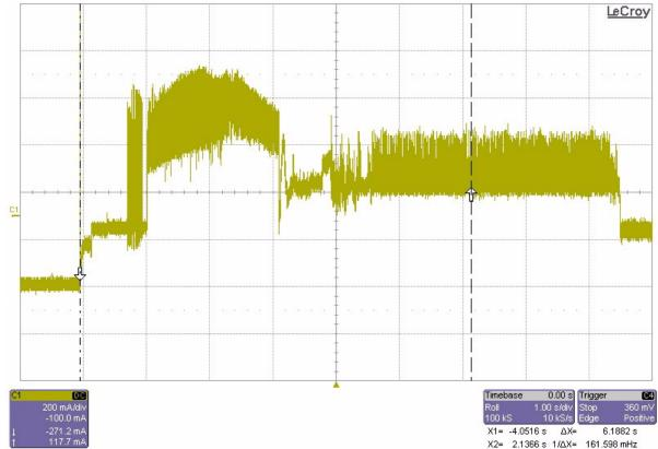
Figure 1. Typical +5V only startup and operation current profile (7200-RPM models)
